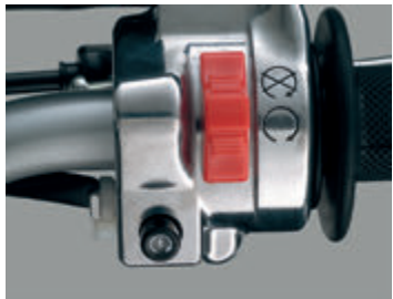
Convenient dual starting system (Push-button electric starter and traditional kick starter) Photo : Electric starter switch
